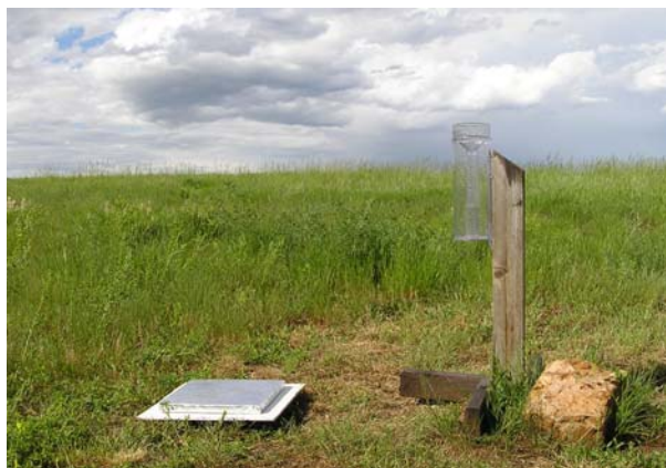
Figure 1. A rain gauge and hail pad at a typical CoCoRaHS volunteer weather station.
