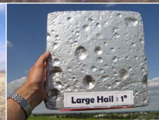
Hail pad = Aluminum foil over a Styrofoam square
