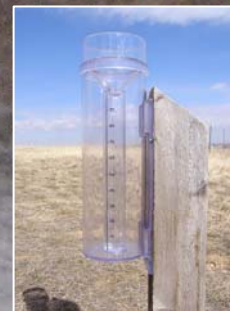
4" diameter high capacity rain gauge holds up to eleven inches of precipitation
