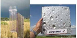
Figure 1. CoCoRaHS Rain Gauge and Hail Pad
