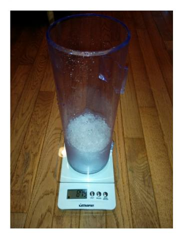
If you are weighing daily snowfall in your **4 inch** precipitation gauge or from a snow core simply place the gauge with contents on your scale and measure the weight in grams:
