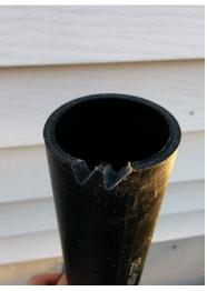
3. Continuing filing until the file reaches it's full depth (top side of the file even with the top of the pipe).
