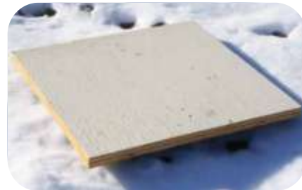
Snow Measuring Board Ex. 16"x16" plywood
