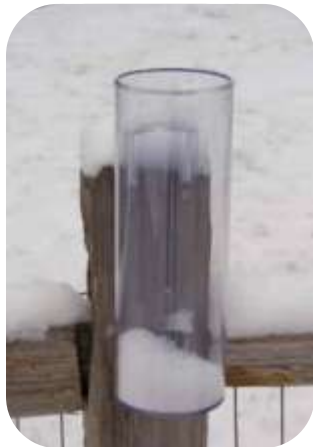
4" CoCoRaHS outer cylinder
