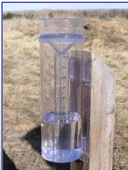
4-inch diameter high capacity rain gauges
