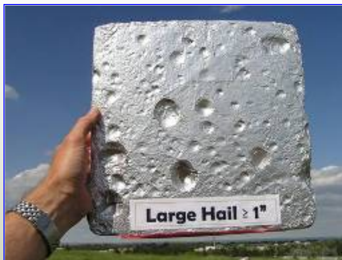
Aluminum foil-wrapped Styrofoam hail pads
