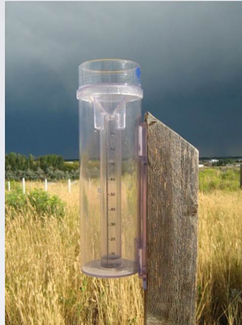
4-inch diameter high capacity rain gauges
