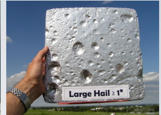
Aluminum foil-wrapped Styrofoam hail pads
