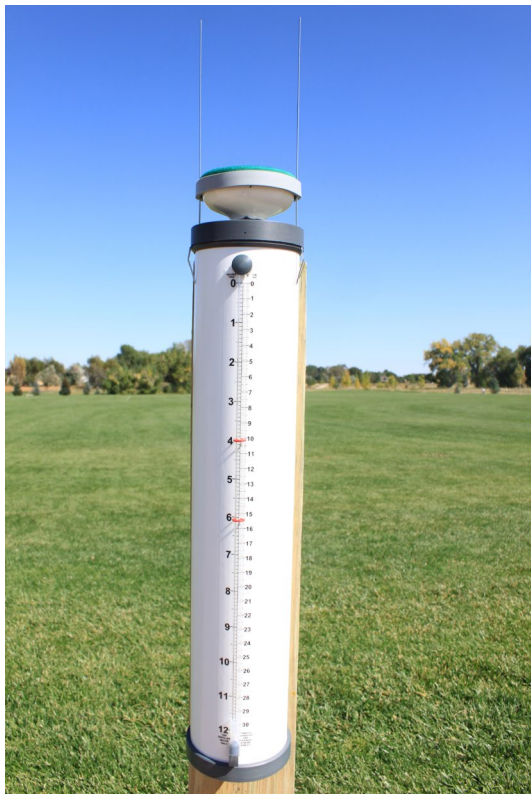
A Reference Evapotranspiration gauge measures the water evaporated from the ground back to the atmosphere both as transpiration from the leaves of plants and also as direct evaporation from open water and soil. This is an optional measurement adopted by the network back in 2012. A handful of volunteer observers take these very helpful supplemental measurements.
