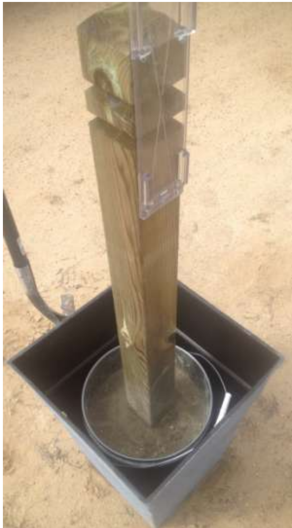
Before: CoCoRaHS Observer CO-WE-387 showing how you can install your rain gauge into a garden planter by using a five gallon bucket!
