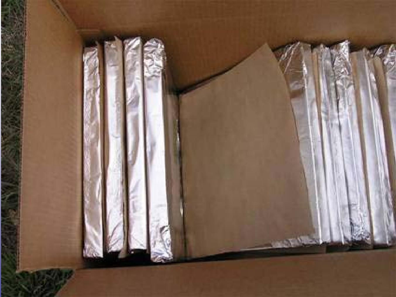
Place your finished hail pads in a box with paper inserted between each pad.
