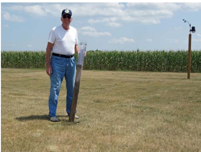
Mike Betourne, IL-KK-23 says the ground has shrunk so much around his rain gauge mounting post that he was able to lift it out of the ground. It is 26 inches deep in the ground and there was hardly any moisture at the bottom of the hole. The post on which his weather instruments are mounted (far right) is also loose in the ground.
