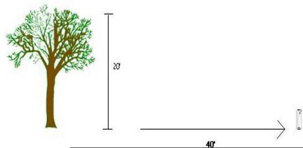
The gauge should be twice as far away from an object as that object is tall. In this picture, the tree is 20 feet tall, so the gauge is 40 feet away.
