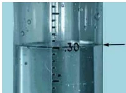
In this picture, we see an illustration of the calibrated measurement tube in the rain gauge that contains three tenths (thirty hundredths) of an inch (0.30 inches)
