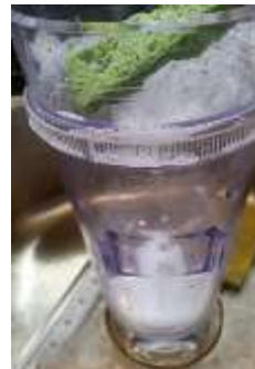
WHILE THE SOAP, WATER AND SPONGE ARE IN USE, CLEAN THE FUNNEL AND OUTER CYLINDER.
