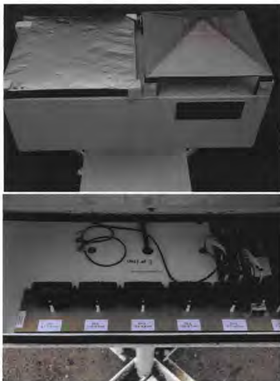
Figure 2. Hail monitor system (HMS): (top) shows hail pad on left and active sensor on right; (bottom) shows the LCD counters for each of the six size channels.
