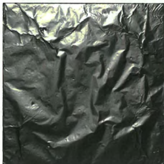
Figure 6. Passive hail pad showing small dents: (top) HM-3; (middle) HM-2; (bottom) HM-1.
