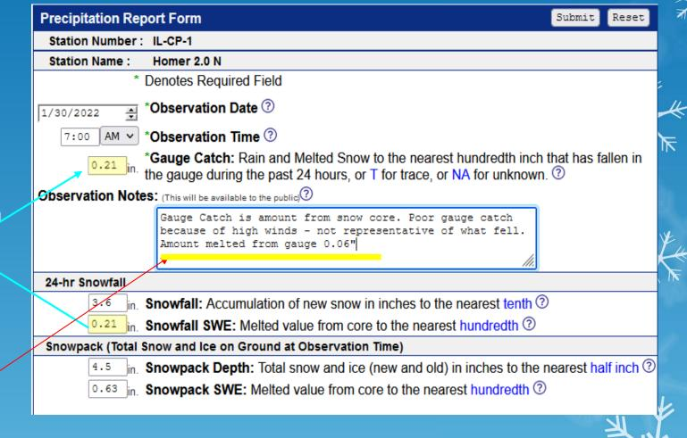
Water melted from core is reported as the Gauge Catch
