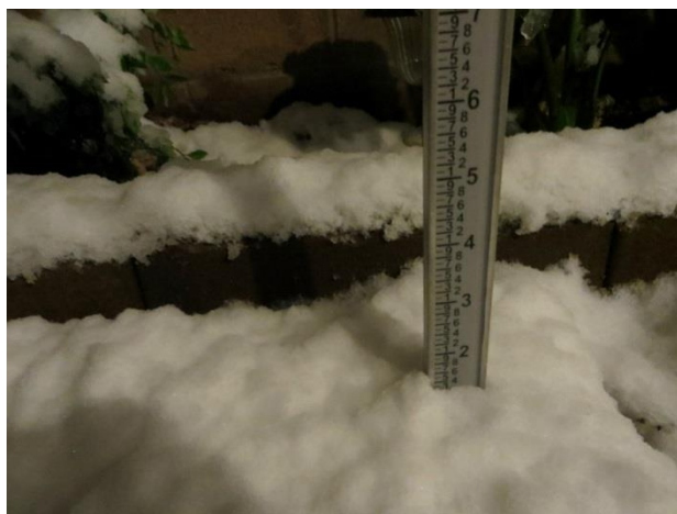
Measuring snow on a snowboard with a snowstick. Photo Credit: NWS Las Vegas.
