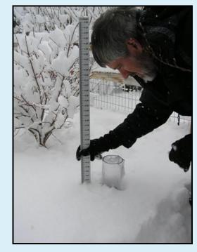
Note that we never measure the depth of the snow in the rain gauge itself. Any frozen precipitation in the rain gauge must first be melted, then measured.
