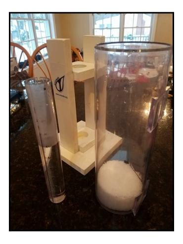
Add a measured amount of hot water to melt the snow in the gauge. Be careful to avoid burns!
