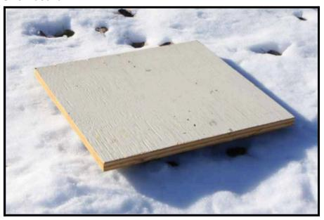
Use a snowboard like this, made of wood and painted white. Place it on a flat surface (not paved), or in an open area away from trees or buildings.
