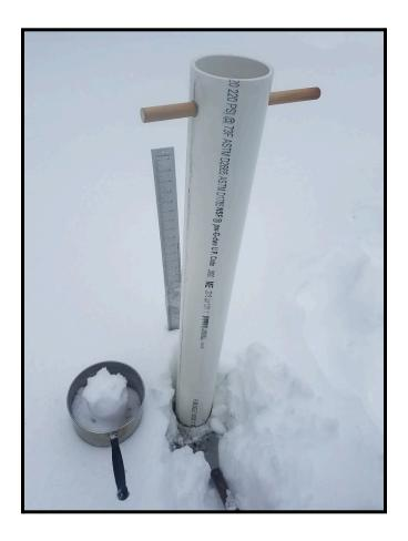
Use a yardstick to measure snow depth. The snow tube can help you get core samples in deeper snow (use the outer cylinder of the gauge for lesser amounts). Put the snow core in a pot (or a bucket) to bring inside to melt.
