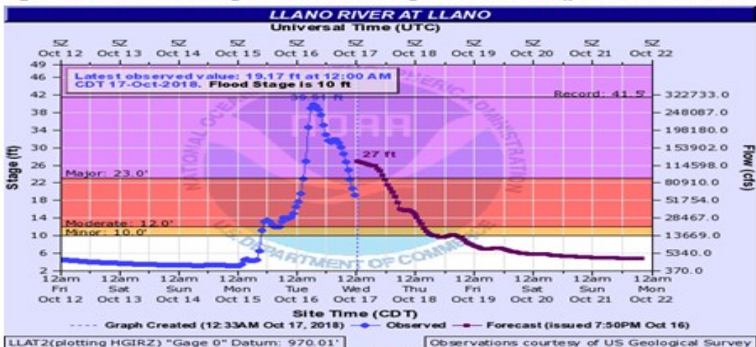
Fig. 5: Llano River at Llano Hydrograph showing crest just below record flood stage
