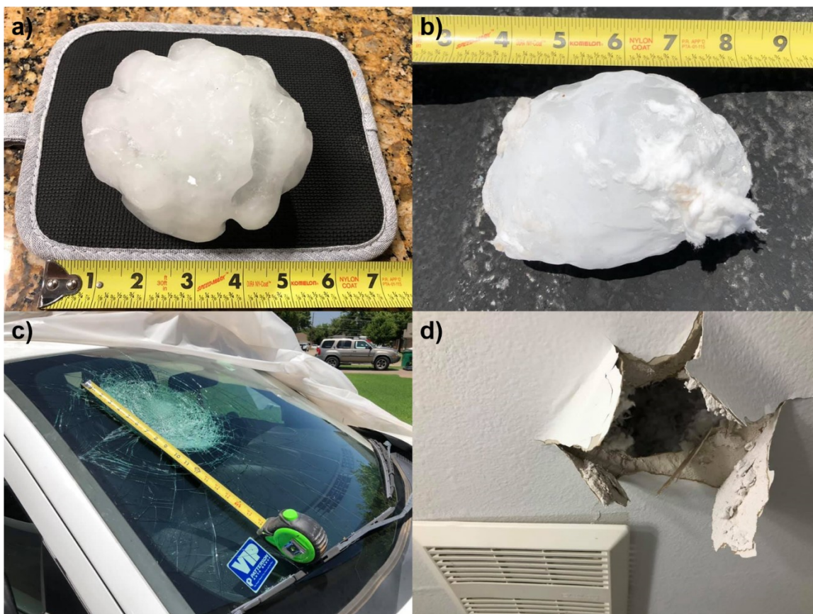
Figure. 1: Pictures of individual hail stones (a and b) and some of the damage they caused (c and d). The hailstone in b) still has some insulation attached to it that it obtained while going through the roof of a home (d). Photos courtesy of Tim Marshall.
