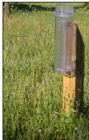
Figure 2: Picture of rain gauge two feet above the ground.
