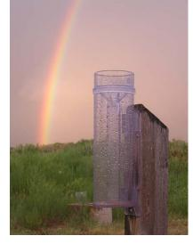
collects in a rain gauge may, in some cases, not equal the amount of precipitation that actually fell. The amount that a rain gauge catches is a function of several variables such as the design and shape of the gauge, its height above ground, the obstacles nearby, wind speed, rainfall intensity, rain drop size, whether the precipitation fell as rain, hail or snow, evaporation
