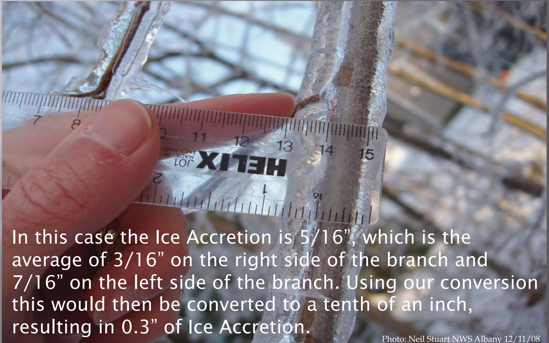
In this case the Ice Accretion is  $\frac{5}{16}$ " , which is the average of  $\frac{3}{16}$ " on the right side of the branch and  $\frac{7}{16}$ " on the left side of the branch. Using our conversion this would then be converted to a tenth of an inch, resulting in 0.3" of Ice Accretion.
