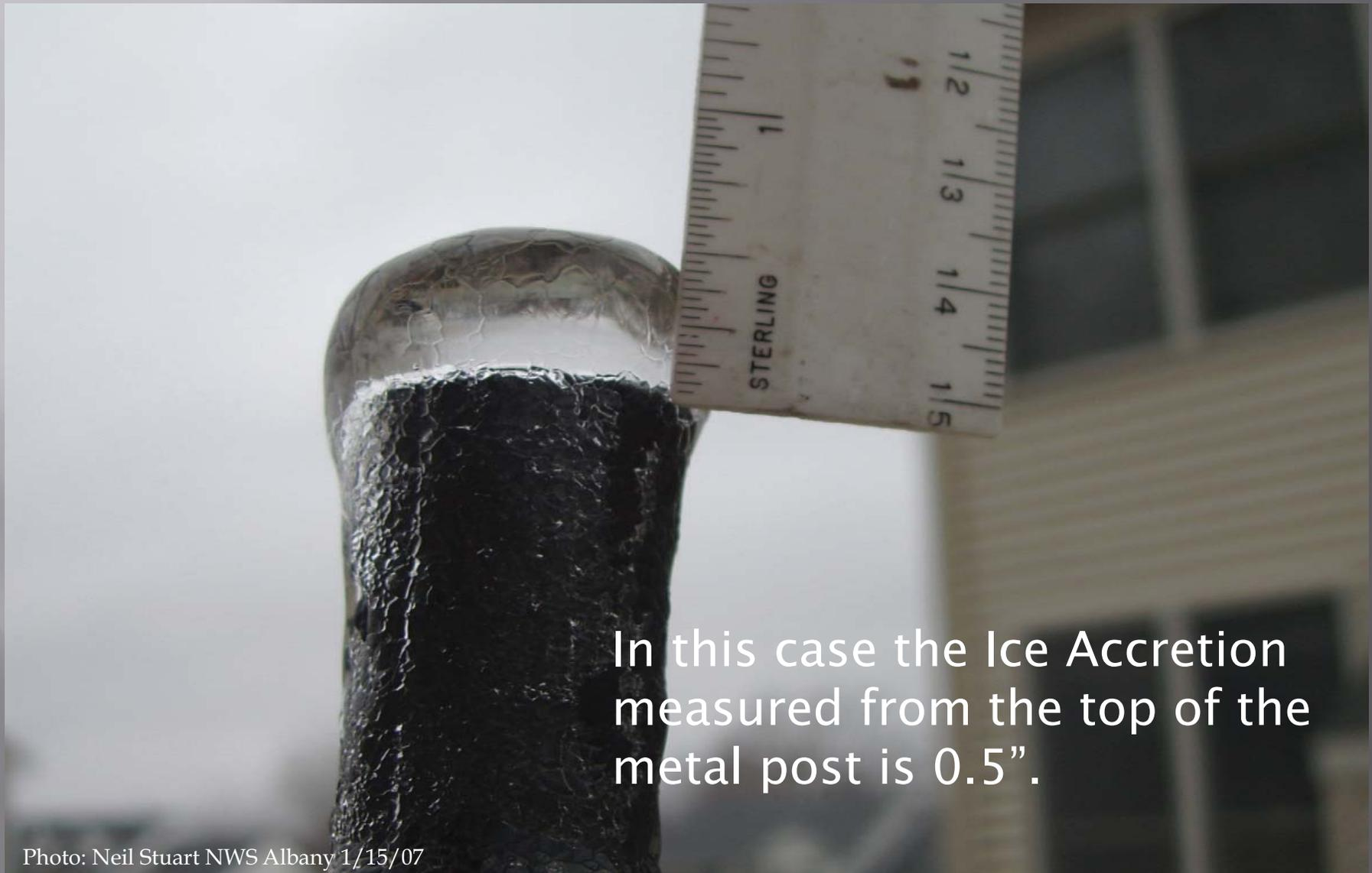
In this case the Ice Accretion measured from the top of the metal post is 0.5”.
