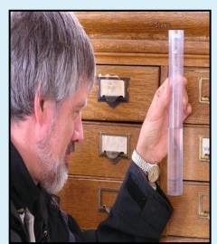
Tube full 0.71- Water added 0.50 = Final reading 0.21
